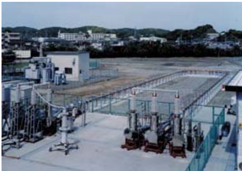
Figure 7. Field test of 114 MVA three-phase HTS cable system, cooled by forced flow of pressurized liquid nitrogen (TEPCO, CRIEPI, SEI)
